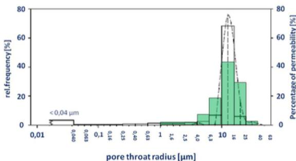
For comparison, the resulting pore throat bins have been plotted within the pore throat radii distribution obtained with mercury injection porosimetry. Figure 3 illustrates the results of both techniques, showing good accordance with each other. GLP measurements “scatter” a little bit more on the flanks of the main pore throat size, which is attributed to the effect of the recalculation for the comparison of both measurements.
