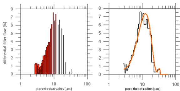
This fitting also allows to recalculate the area underneath of the fitting curve to the same bin sizes used for the mercury experiment (right hand side).
