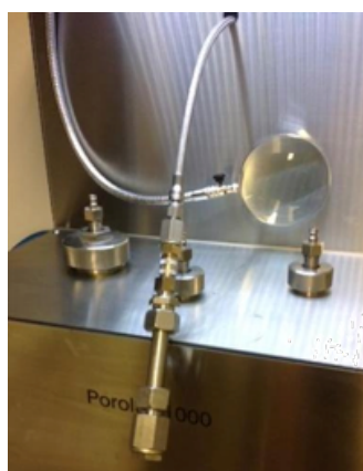
Figure 3: SHHF attached to the POROLUX™ 1000 for outside-in measurements.
