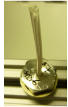
Figure 7: multiple fibres glued together.
