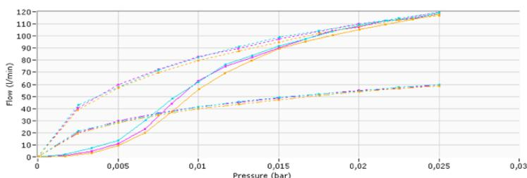
Figure 2: Wet, dry and half dry curves for material A
